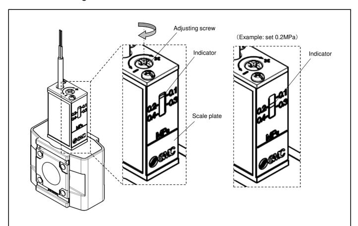
Pressure is adjusted by rotating the adjustment screw and setting the indicator to the figure on the scale. Set pressure increases by rotating the adjustment screw clockwise. Use a screwdriver of a size suitable for the groove (+) of the adjustment screw.
