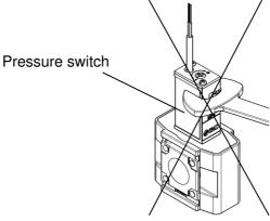
(5) Do not apply torsion or bending moment other than the weight of the product itself. External piping needs to be supported separately as it may cause breakage. Non-flexible piping like steel tube is susceptible to excessive moment load or vibration. Insert flexible tubes to prevent this.
