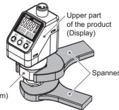
When tightening, do not hold the upper part of the product (Display) with a spanner.
