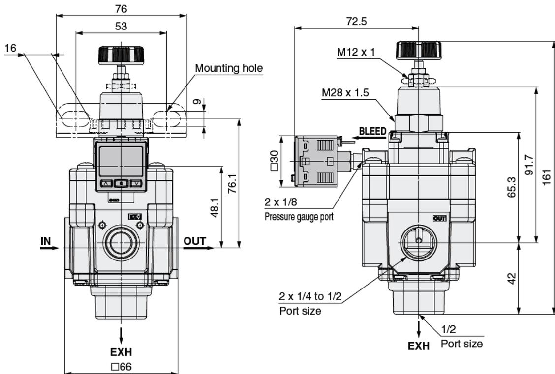
8-2. Dimensions of the regulator with the front or back exhaust direction [IR30\*(1, 2)-A].
