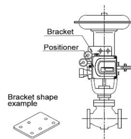
Attach using the screw hole at the positioner back and the screw hole at the front mount of diaphragm valve.
