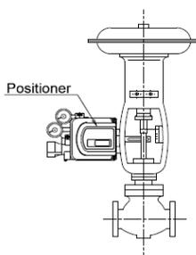
Directly attach using the screw hole at a side of the positioner and the screw hole at the yoke side of diaphragm.
