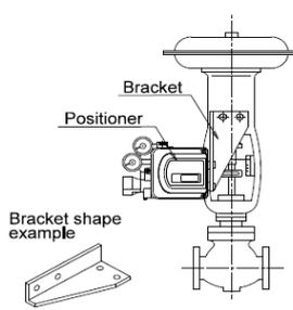
Attach using the screw hole at a side of the positioner and the screw hole at the front mount of diaphragm valve.
