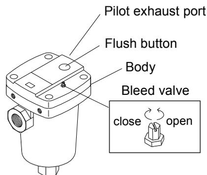
[Disassembly and cleaning of auto drain]
