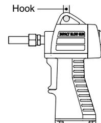
9. When the blow gun is used or stored, confirm that no twisting, turning, or tensile force or moment load is applied to the port or tube. This may cause fittings to fracture or tubes to be crushed, burst, or come loose.
