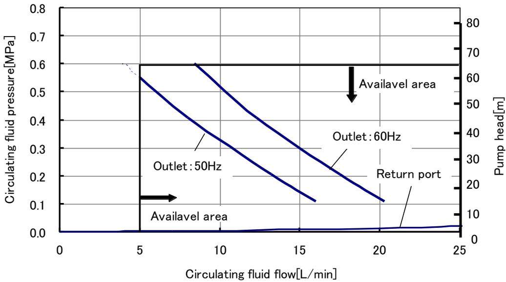
Fig. 9-9 Pump capacity(HRS030-\*\*-20-MT)
