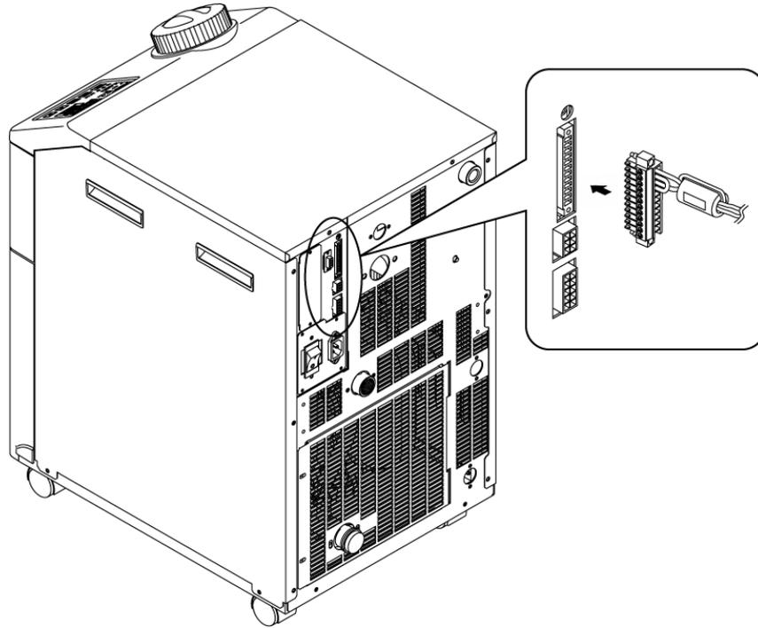
Fig. 3-8 Connecting the Remote control signal cable
