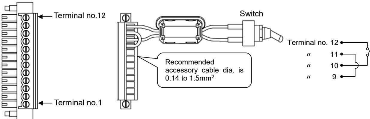
Fig. 3-7 Wiring of contact for remote signal inputs (Example)
