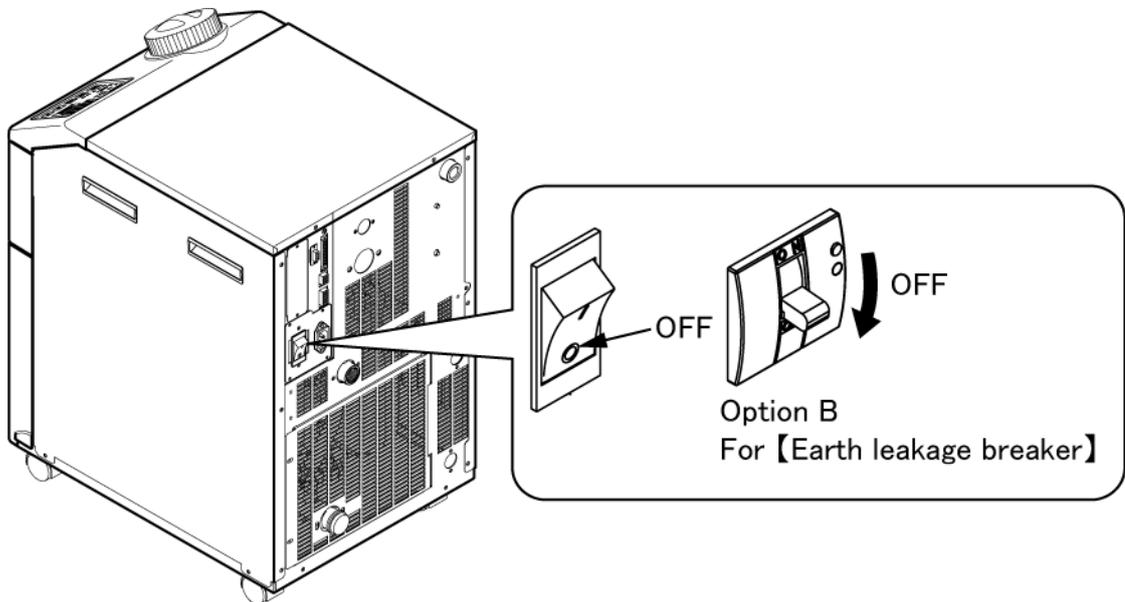
Fig. 1-4 Location of the switch for the power supply
