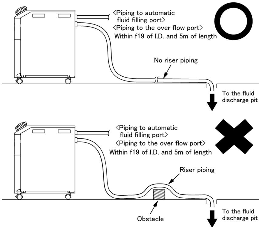
Fig. 3-14 Piping to automatic fluid filling port and overflow port
