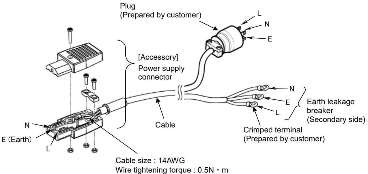
Fig. 3-5 Power supply cable
