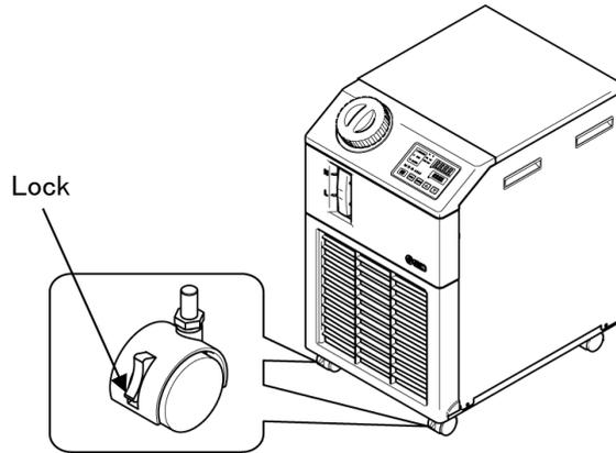
Fig. 3-3 Installation procedures
