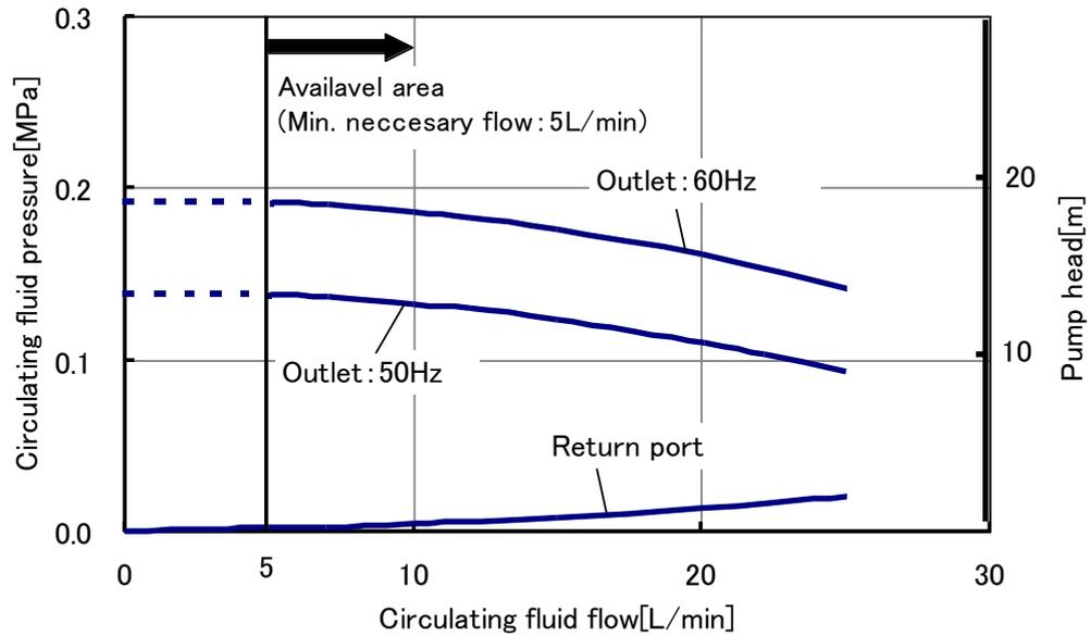
Fig. 9-7 Pump capacity(HRS030-\*\*-20-(BJM))
