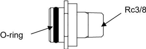
Fig. 8-7 Fitting for the drain port (Accessories)
