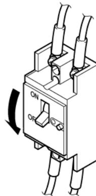
Fig. 1-5 Shut off of facility power supply
