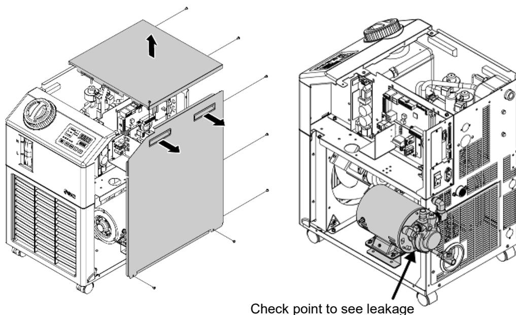
Fig. 8-3 Check for water leakage from pump
