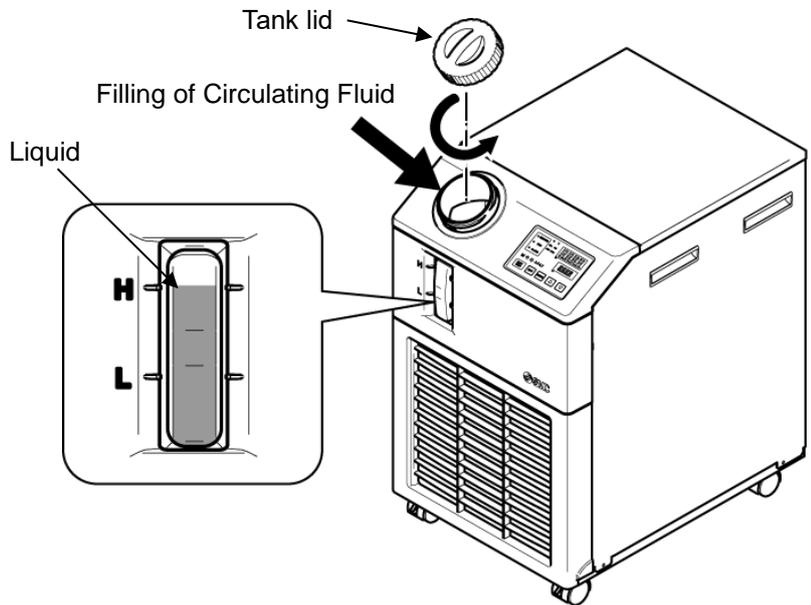
Fig. 4-6 Filling of Circulating Fluid
