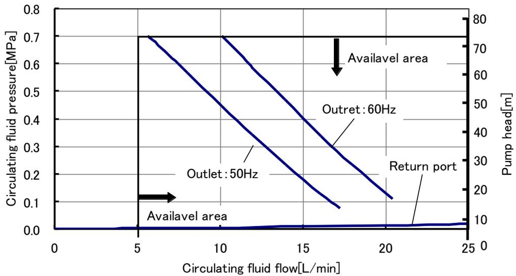
Fig. 9-8 Pump capacity(HRS030-\*\*-20-T)
