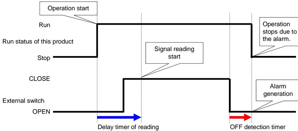
Fig 3-15 Timing chart of external switch monitoring
