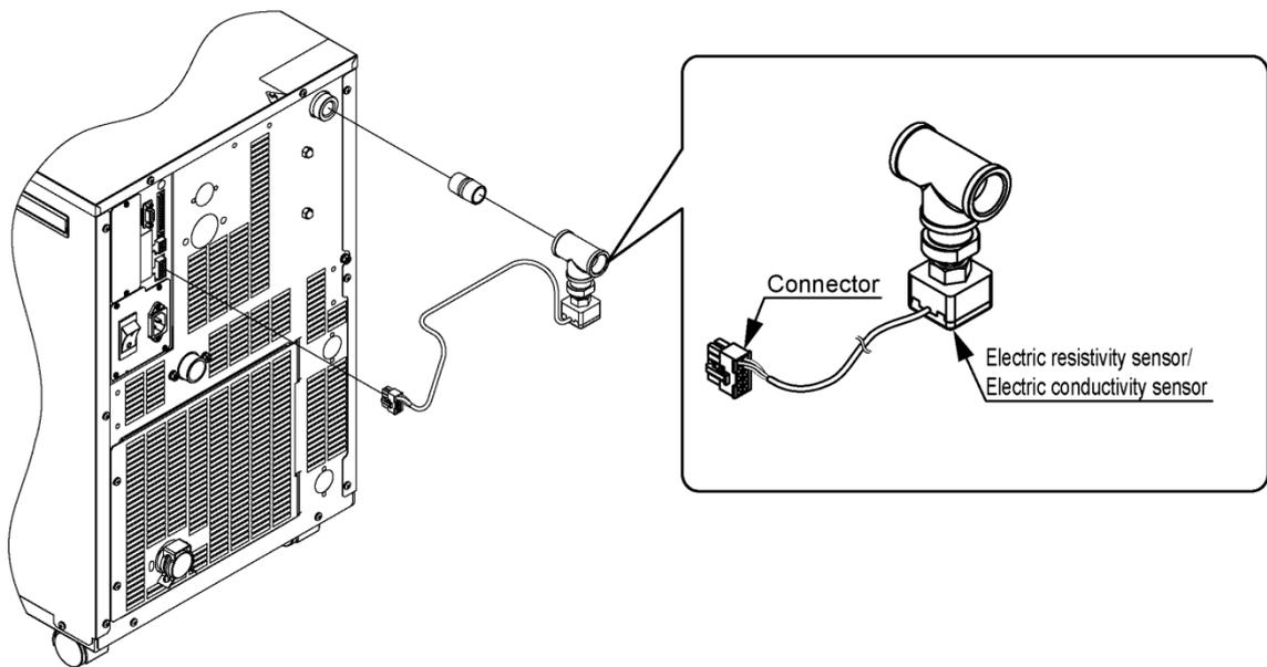
Fig 6.4-1 Optional Accessories [Electric resistivity/conductivity sensor set]
