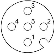
BUS IN: M12 5-pin plug, A-coded
