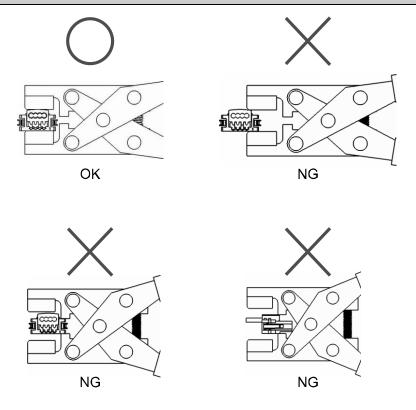
(3) After attaching the cable, confirm that it is properly pressure-welded.
