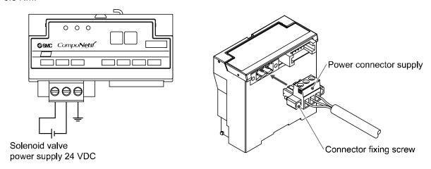
Applicable cable of the power supply connector
