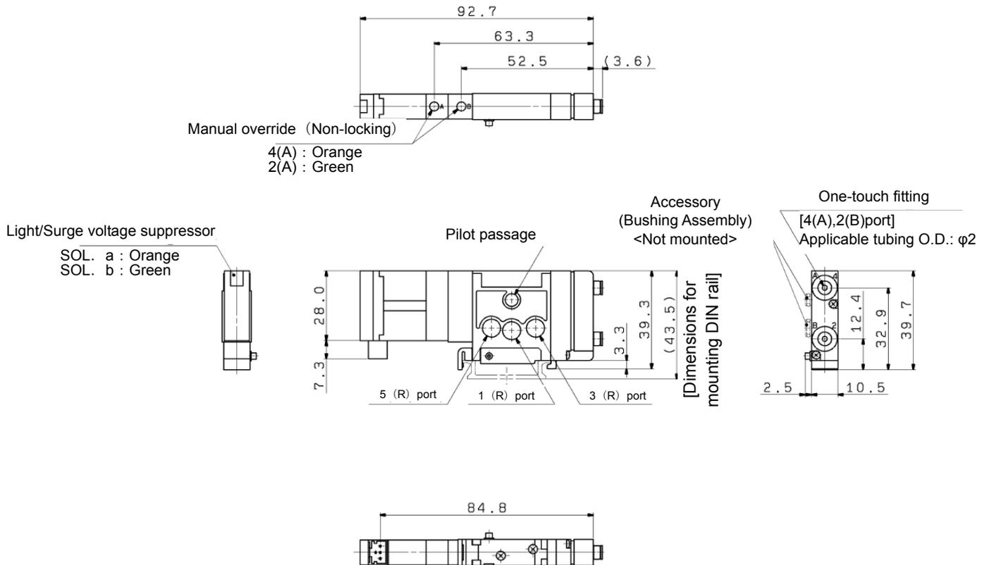
Note: The illustrations show the SZ3260-5LOZ-C2-X84 model. The dimensions other than the A, B port sizes are the same as the standard model.
