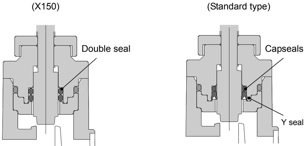
\* Reduce the liquid leakage issue when circulating fluorine liquid.
