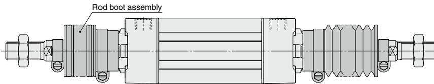
\* Replaceable with the rod boot assembly
