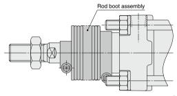
\* Replaceable with the rod boot assembly For details on replacement part numbers, refer to page 248.
