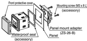
Tighten screws 1/4 to 1/2 turn after the heads are flush with the panel.
