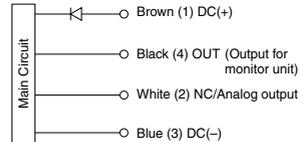
\* Use this sensor by connecting it to a SMC remote type display unit, Series PF2W2□□/3□□.
