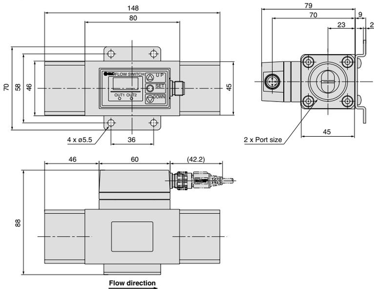
**Dimensions: Remote Type Sensor Unit For Water**
