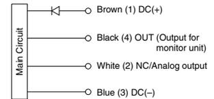
\* Use this sensor by connecting it to a SMC remote type display unit, Series PF2W3□.
