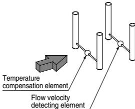
This flow switch uses L/min as the flow rate indicator unit. The mass flow is converted and displayed under the conditions of 0°C and 101.3 kPa and 20°C and 101.3 kPa.
