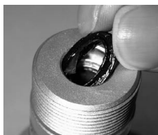
Picture 6: Installation of rod seal
