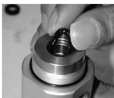
Picture 7: Installation cushion seal
