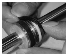
Picture 8: Installation of piston seal
