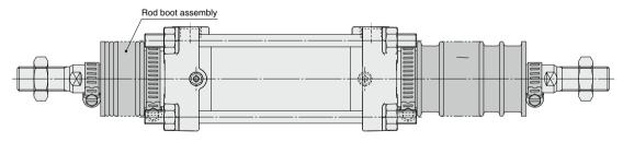
\* Replaceable with the rod boot assembly For details on replacement part numbers, refer to page 248.
