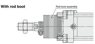
Replaceable with the rod boot assembly For details on replacement part numbers, refer to page 248. (CA2 only)
